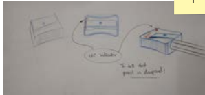
When the sharpened point touches the push switch a little, the red led indicator blinks.
